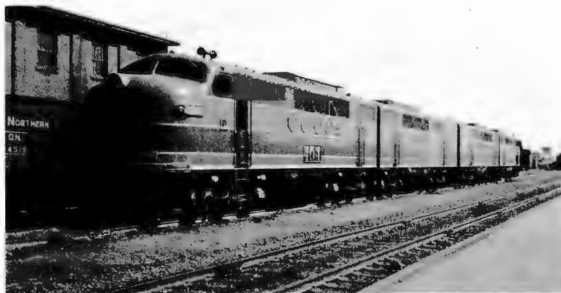
G.N. 404 Freight Diesel A-B-B-A 4 units 0-B-B-0 1 unit Dynamic Breaking 193' long 15' high 10'2" wide 460 tons total wt. Built by EMC 1944 Hillyard 7-?- 44 (Author's Collection)
