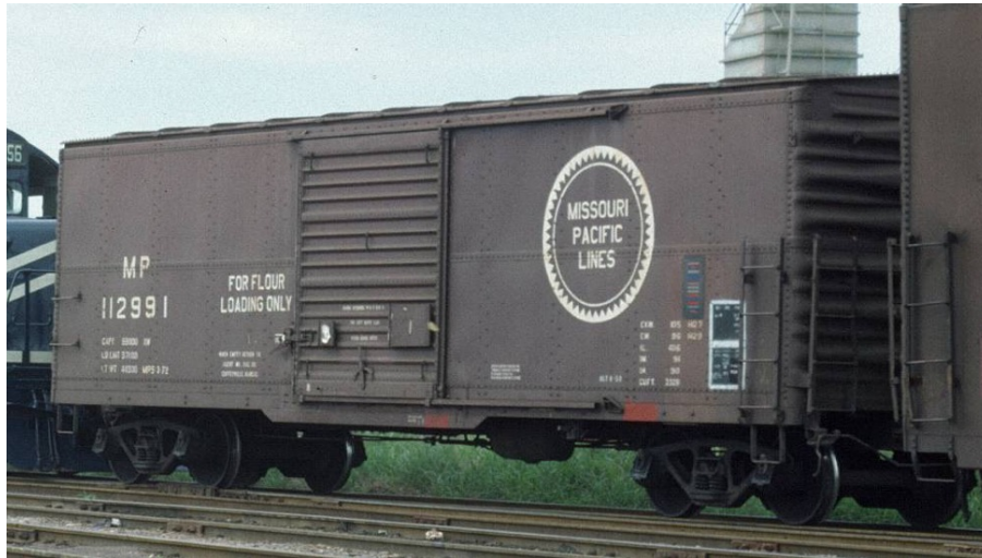
MP 112991 in flour loading assignment. Car shows COTS stenciling and the ACI label. The cut down side and end ladders were only on the 'A' end of the car.
